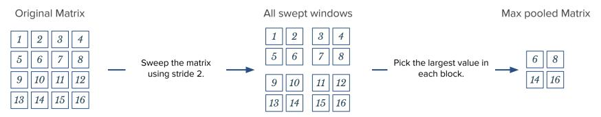
Max-pool layers are used to downscale the input by extracting the most important feature.
